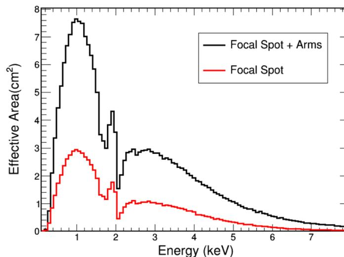
Figure 3-2: Simulated effective area curves of WXT for the central focal spot (red) plus the cruciform arms (black). The pores are coated with Iridium, which produces the absorption edge seen at  $\sim 2$  keV. The response of the detectors, coated with a 200 nm-thick Aluminum layer, is incorporated.
