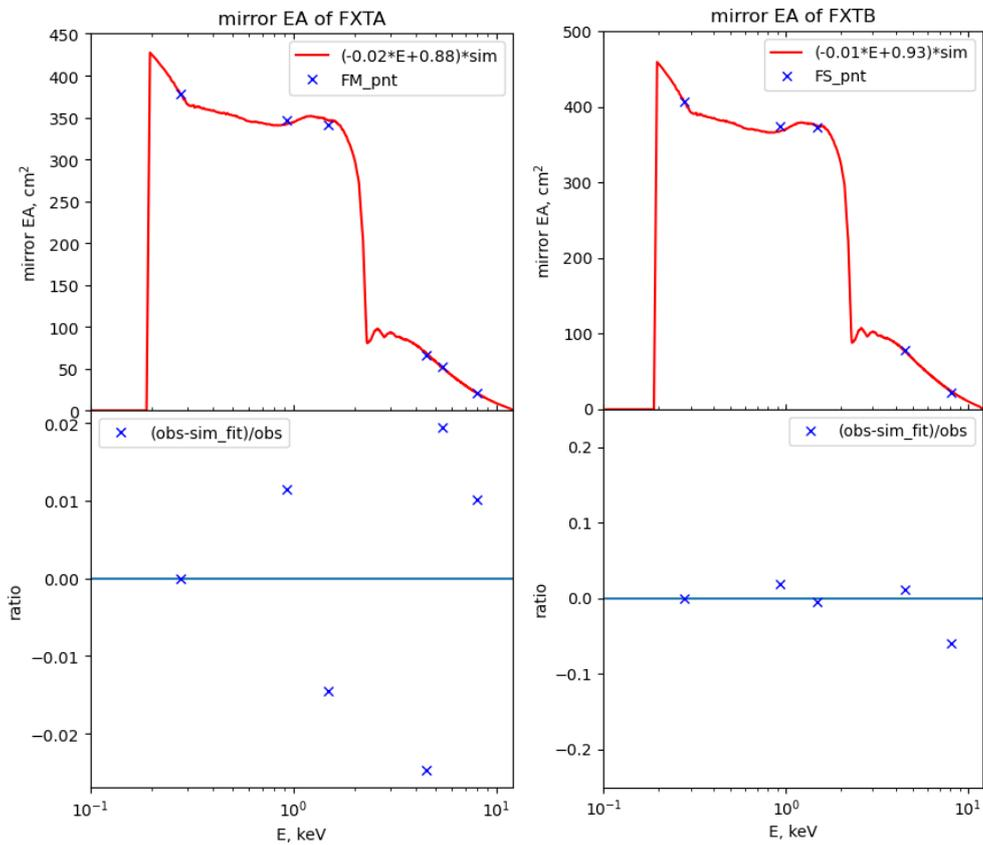
Figure 4-15: The effective area of the mirror assembly
