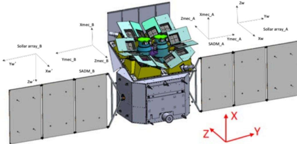
Figure 2-2: the definition of satellite coordinates and axes.
