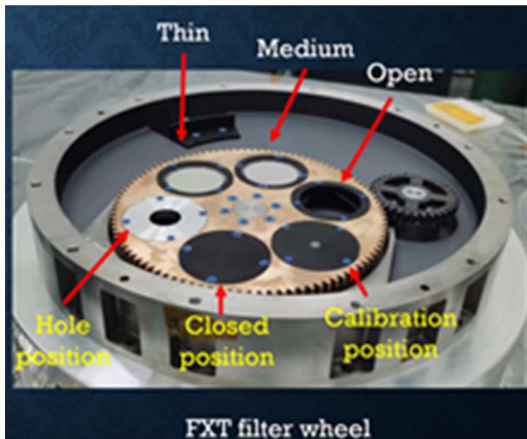
Figure 4-12: The filter wheel of FXT
