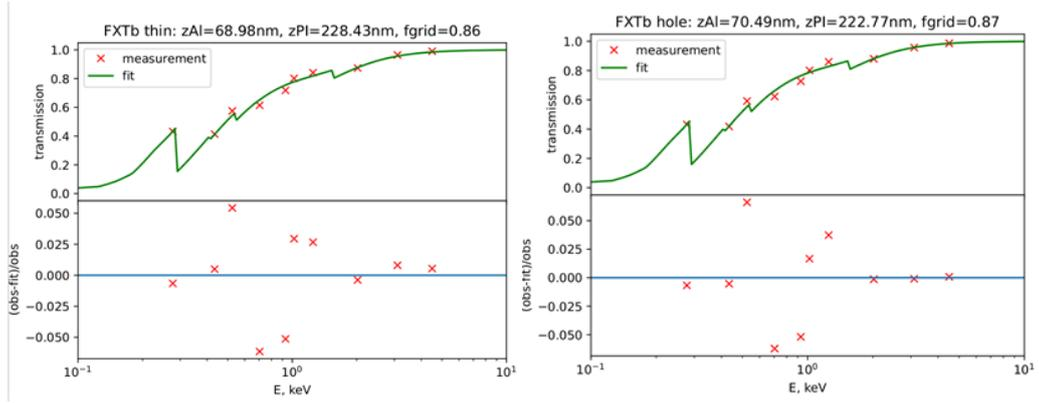
Figure 4-14: The transmission curve of FXT filters
