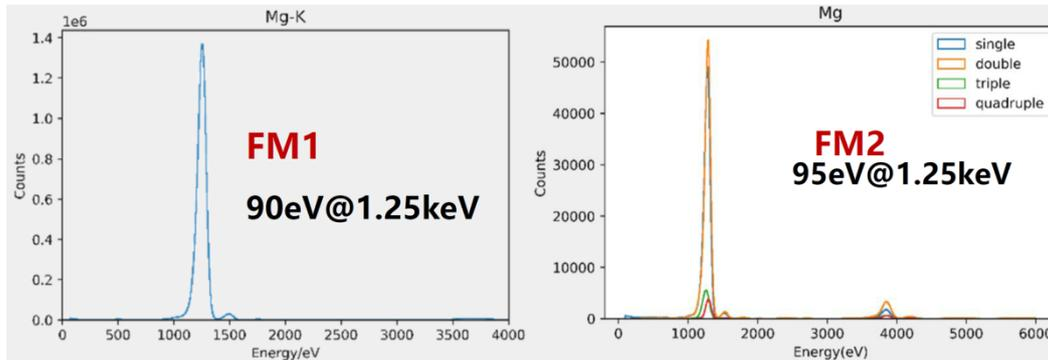
Figure 4-5: FXT energy resolution at 1.25 keV.
