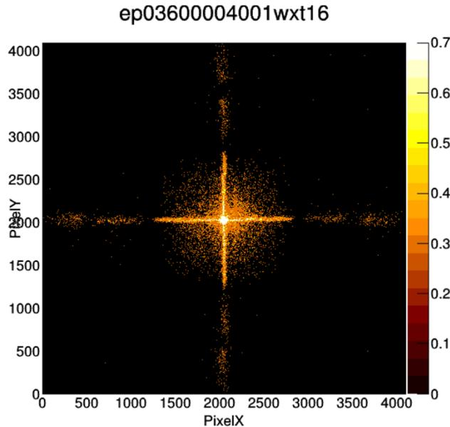
Figure 3-4: True X-ray image produced by one mirror assembly qualification model of the WXT module developed at NAOC (measured at MPE/Panter by using a parallel beam of a Cu-L $\alpha$  line source of 930 eV). The PSF is symmetric, with an angular resolution  $\sim 5$  arcmin in FWHM for the central spot. (Courtesy ESA/MPE)
