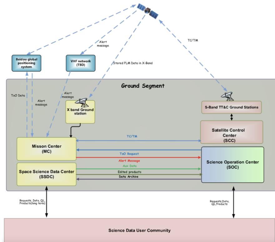
Figure 5-1: Sketch of EP data and information flows and the ground segment
