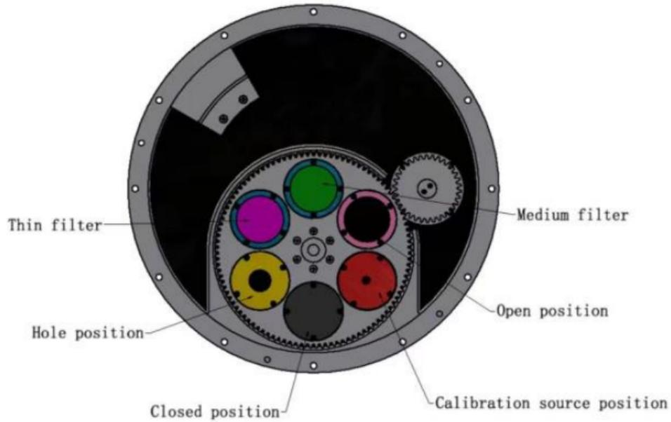
Figure 4-2: The filter wheel of FXT
