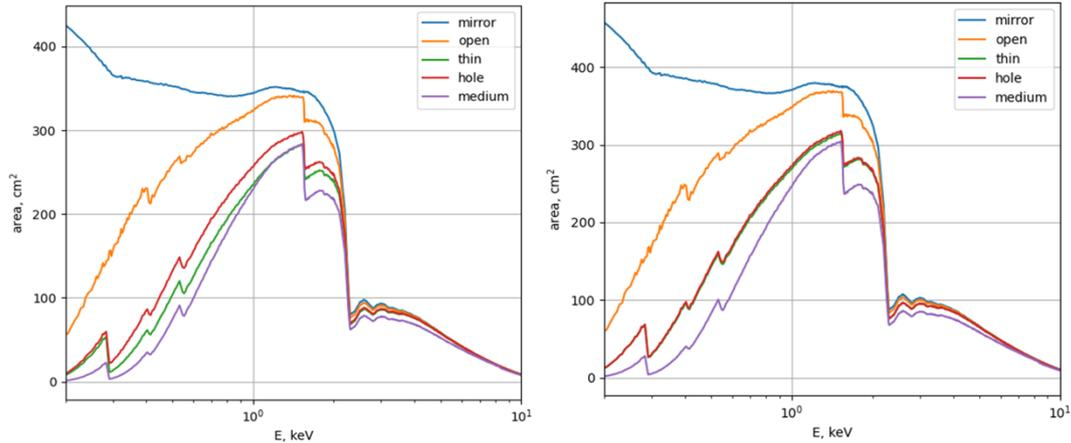
Figure 4-16: The effective areas of FXTA (left) and FXTB (right)
