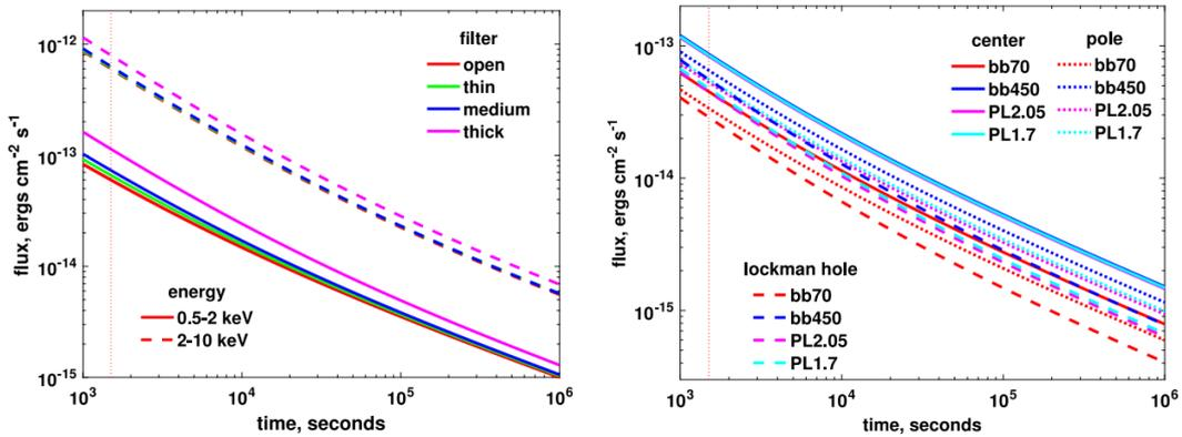
Figure 4-9: The estimated sensitivity of one EP/FXT module.
