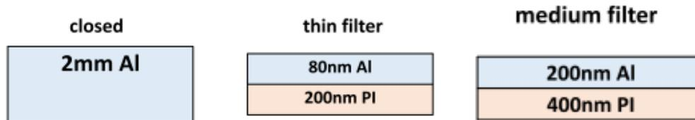
Figure 4-13: The designed geometries of FXT filters
